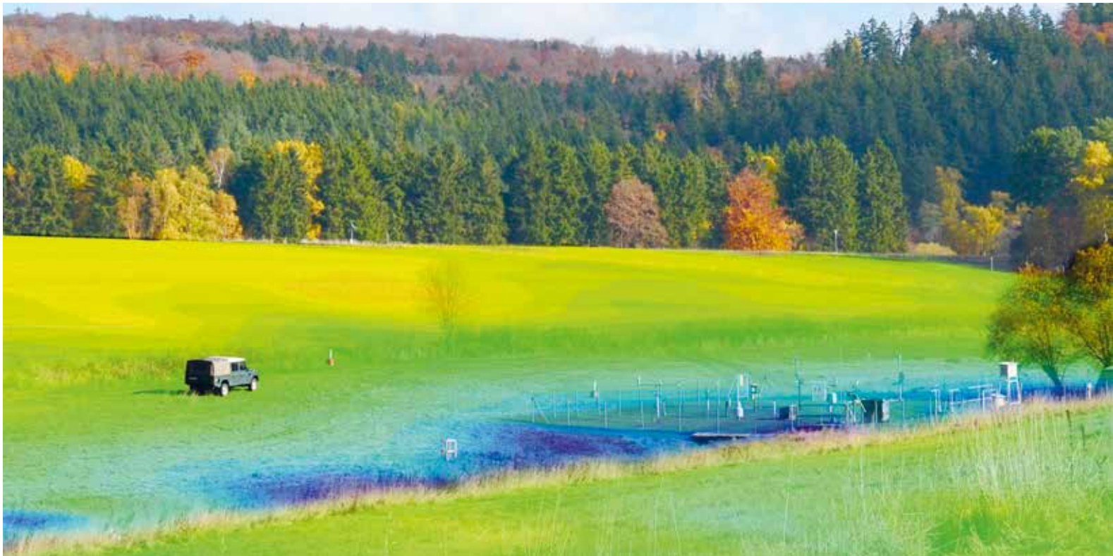
The cosmic-ray measuring device in the boot of the UFZ Land Rover can gauge the soil moisture in a 150-m radius and down to a depth of 50 centimetres.
