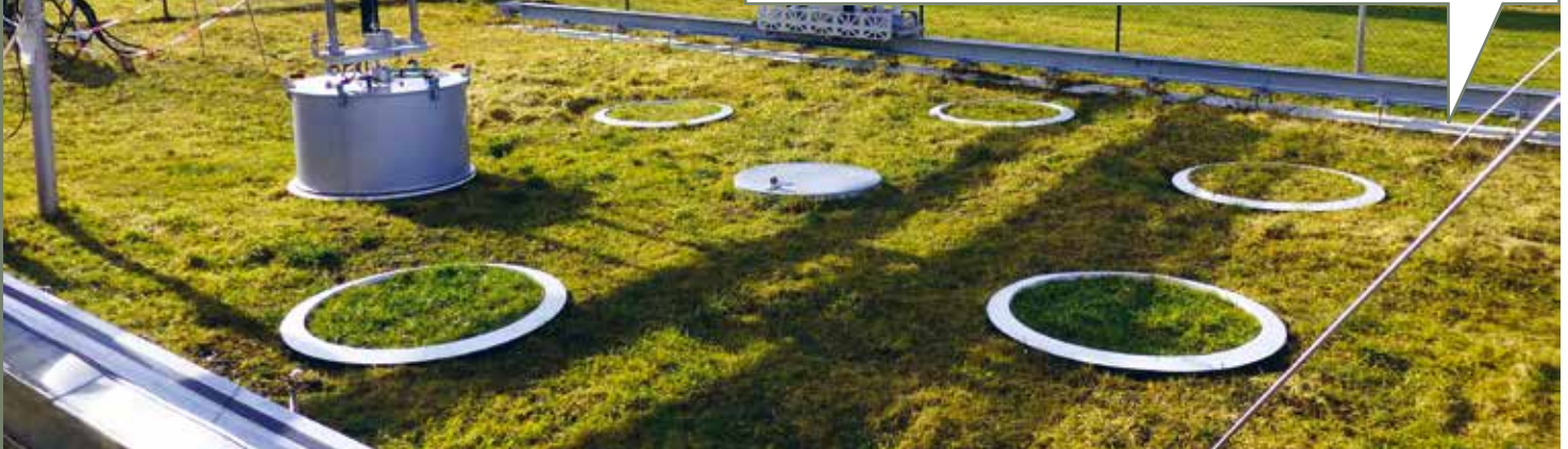
At the TERENO observatory in Fendt, robots assess soil columns from different elevations to determine which greenhouse gases their microorganisms are releasing.
