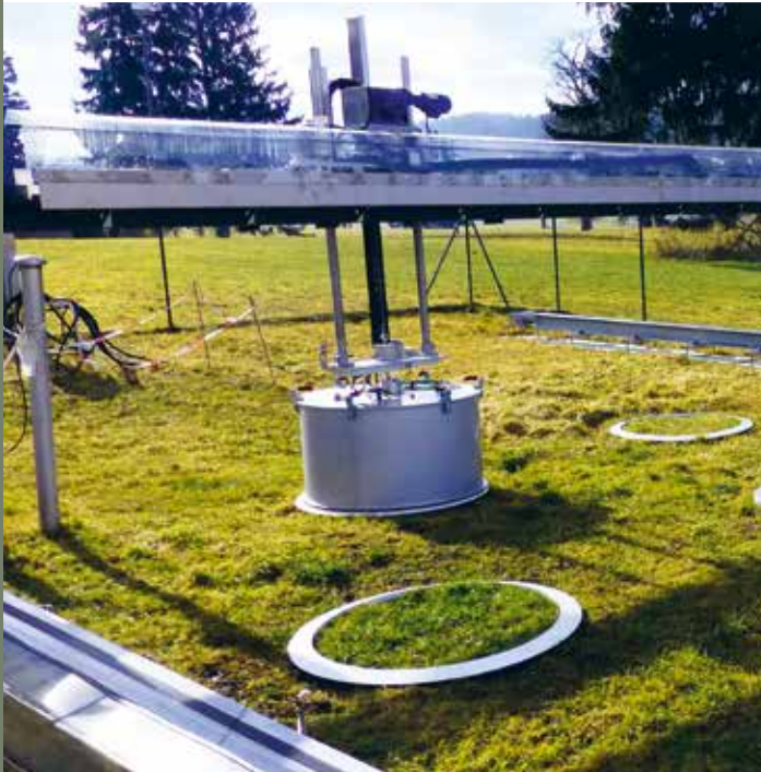
At the TERENO observatory in Fendt, robots assess soil columns from different elevations to determine which greenhouse gases their microorganisms are releasing.
