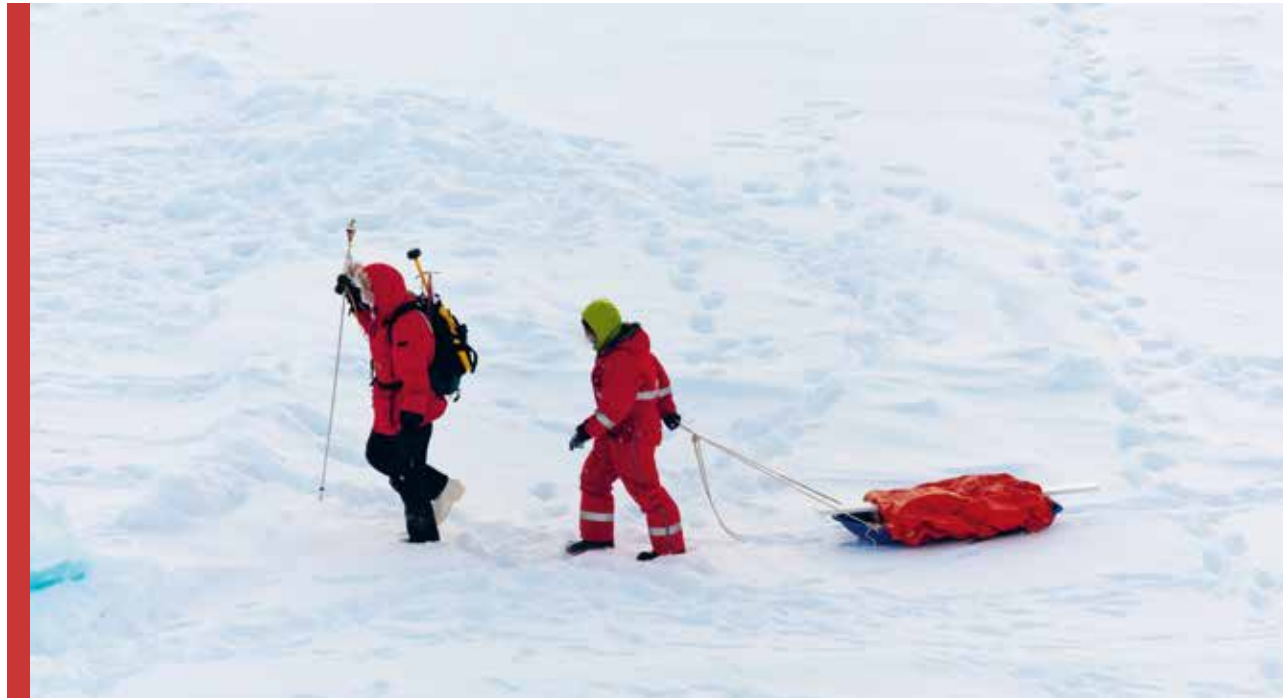
On a level and undeformed part of the floe, measuring the ice thickness is a fairly straightforward task: one researcher walks ahead and measures the snow thickness with the so called MagnaProbe. The second follows, dragging the measuring sledge behind them.
