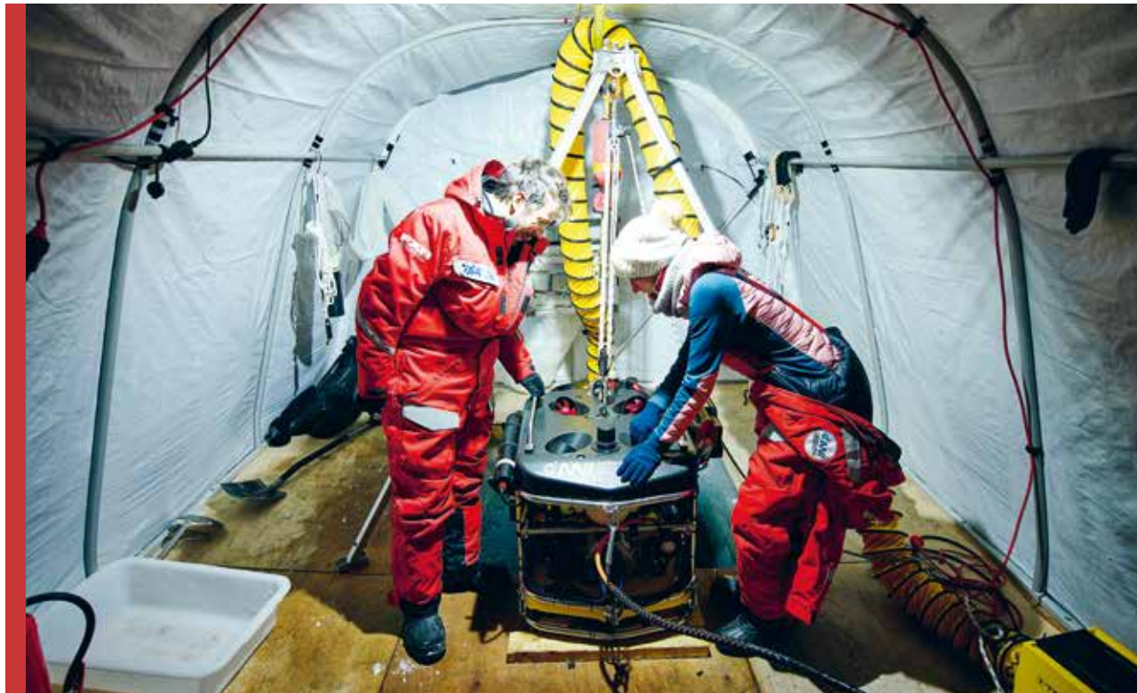
The AWI's ROV is hardly a lightweight: it takes the muscle power of two researchers to lower it into the water through the entry hole. A tent that was erected over the hole protects the sea-ice physicists from the wind and snow.
