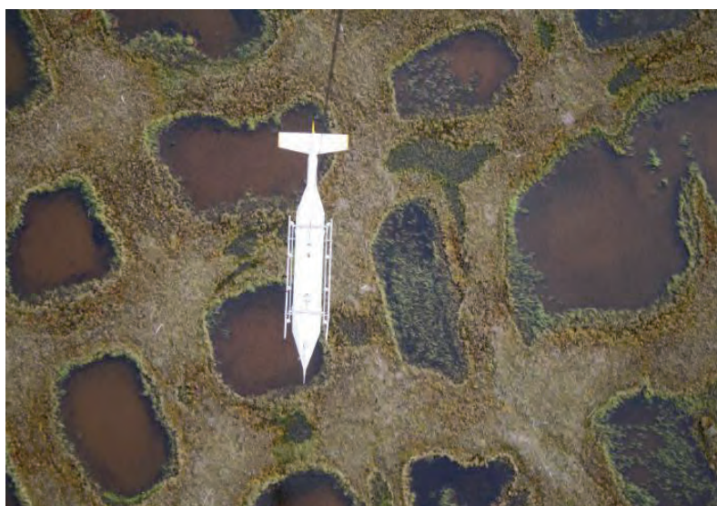
Fig. 3.4: The helicopter towed sensor "Helipod" during measurement of turbulent heat and CO 2 fluxes over the Siberian Lena Delta. (Photo: Torsten Sachs, GFZ)
