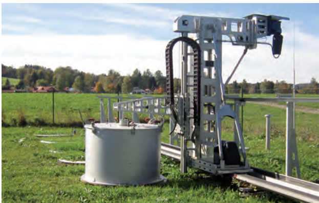
Fig. 4.1: Automatic greenhouse gas measuring system at TERENO location in Rottenbuch. (Photo: Ralf Kiese, KIT IMK-IFU)
